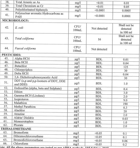
Note: All the above parameters are tested as per APHA methods, 23<sup>rd</sup> Edition, 2017 BDL- Below detectable limit, Detectable limit- <0.005 µg/l
